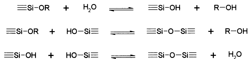
Fig 1. Hydrolysis and condensation of TEOS [2]
